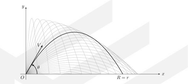
Given a gravitational acceleration of  $gm s^{-2}$ , the displacement vector of a projectile with angle of projection  $\theta$  and velocity  $Vm s^{-1}$  can be shown to be
